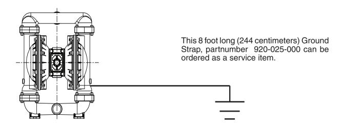
To reduce the risk of static electrical sparking, this pump must be grounded. Check the local electrical code for detailed grounding instruction and the type of equipment required, or in the absence of local codes, an industry or nationally recognized code having juristiction over specific installations.
