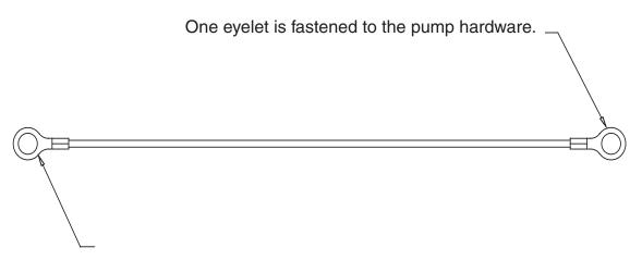
One eyelet is installed to a true earth ground.
