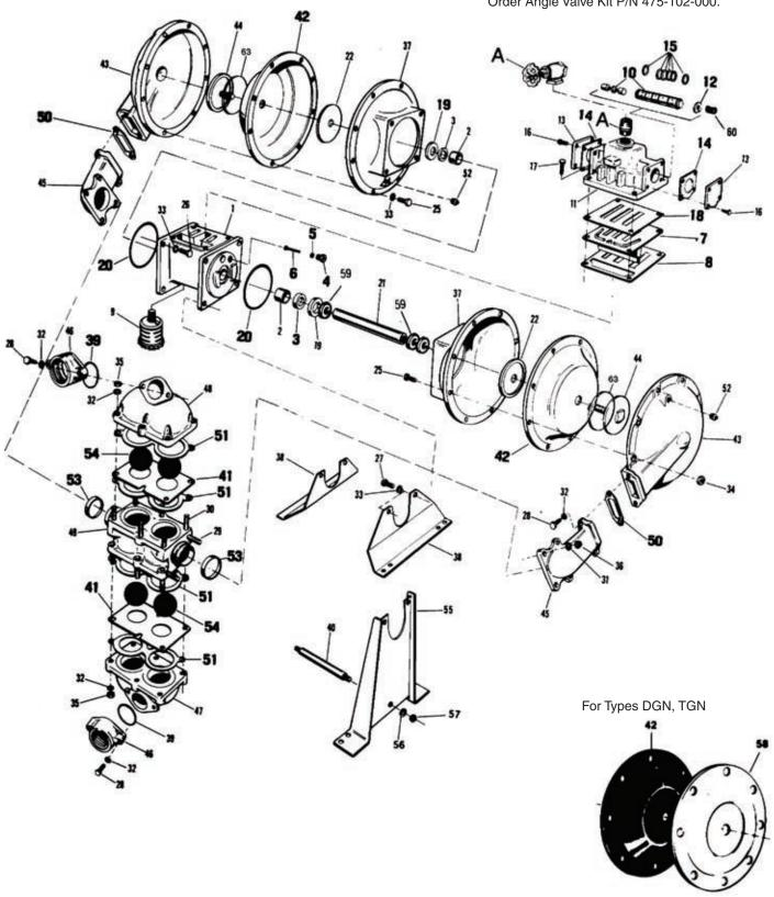
Ribs on Virgin PTFE Diaphragm are to be toward the pumping material.
