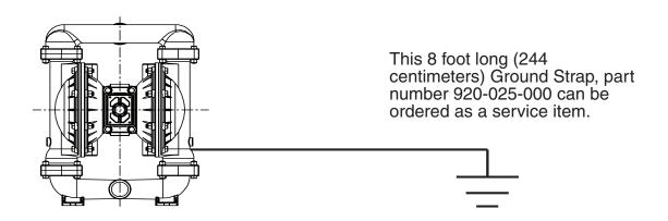
To reduce the risk of static electrical sparking, this pump must be grounded. Check the local electrical code for detailed grounding instruction and the type of equipment required, or in the absence of local codes, an industry or nationally recognized code having juristiction over specific installations.
