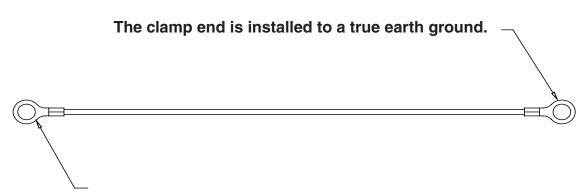
The eyelet end is fastened to the pump hardware.
